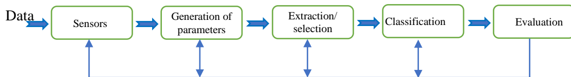
Fig. 1 The process of pattern recognition
